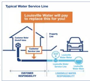
The service line is the pipe that brings drinking water from the water main into your home. Louisville Water installs a service line from the water main and the customer installs one on their property. Older homes (those typically built before 1950) may still have a lead or galvanized service line.
